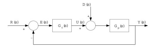
Fig. 1. System block diagram for pitch mode control of a small aircraft.
