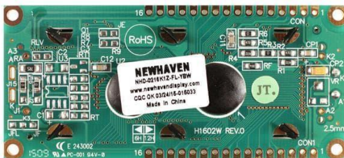
Fig. 4: Newhaven Display LCD Character Display NHD-0216K1Z-FL-YBW
